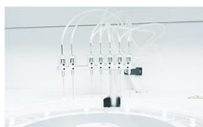
Washing Probe Independent 7-step washing system.
